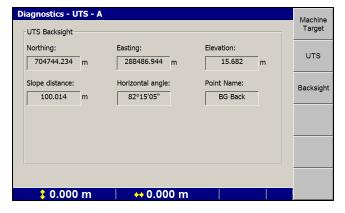
This screen displays information about the backsight taken to establish the orientation of the UTS instrument. The fields within this screen are explained below.
