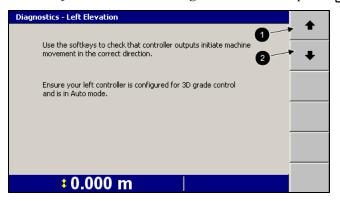
Note - The above image shows an example of the left elevation controller outputs dialog.
