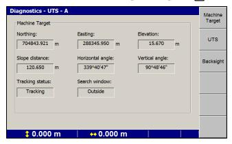
The first Diagnostics – UTS screen is Machine Target. This is the screen that appears if you press Machine Target. The fields in this screen are explained below:
